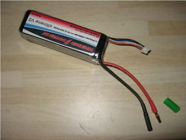
This way, they can't be connected with reversed polarity. You will also note that I use a piece of silicon tube to cover the bare male connector when not in use.
